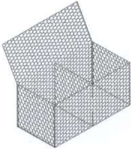
River bank protections with gabions manufactured with double twisted steel wire mesh. Gabion units are filled with stones integrated with live plants using bio-engineering techniques.
