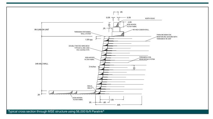
The MSE structures not only retained North Road, but also provided erosion control and training works for the river channel at the foot of the structures. Terramesh® structures can accommodate large differential settlements without sustaining damage. This is a crucial capability in channeling works, where erosion can cause settlement.
